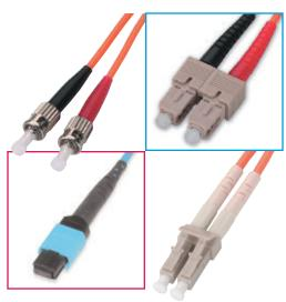
Signamax offers a comprehensive line of optical fiber patch cords for cross-connect or work area applications. Patch cords are available in simplex or duplex, multimode (62.5-µm or 50-µm) or single-mode with ST, SC and small form factor connectors including LC and MT-RJ. Patch cords are manufactured using OFNR riser grade cable and are 100% factory tested to ensure performance to ANSI/TIA-568-C.3 standards.
